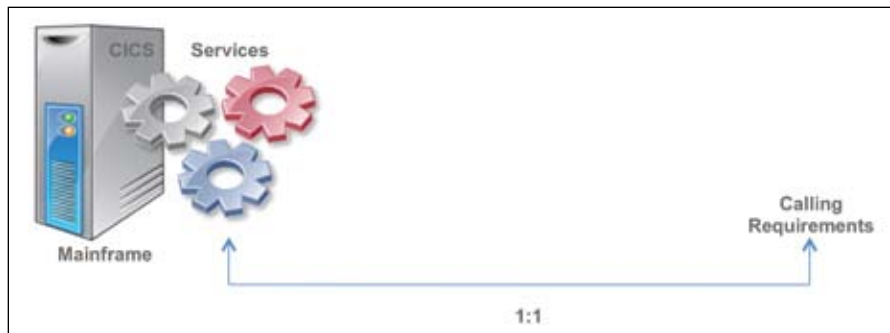
This one-to-one access approach lets a client application call a service, which can create a direct, authenticated link with the destination CICS application to perform the interactions.
